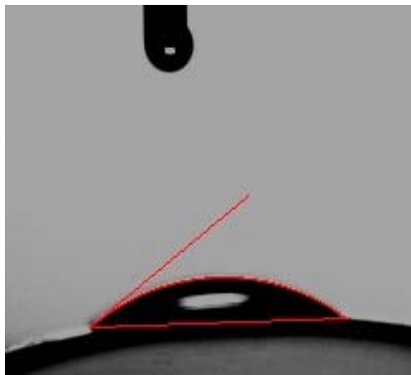
Figure 1. Drop of saline on an untreated lens. Figure 2. Drop of saline on a plasma treated lens
